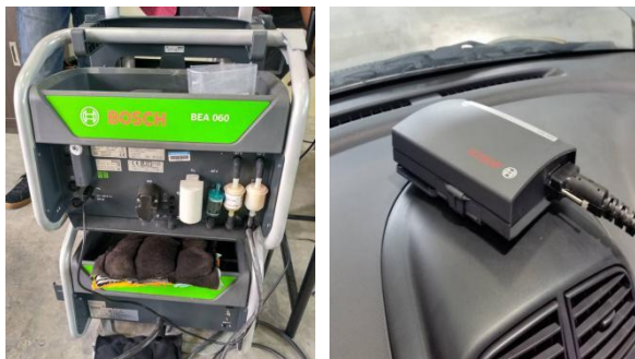
Fig. 2 - Bosch Emission Analyzer & KTS 515
